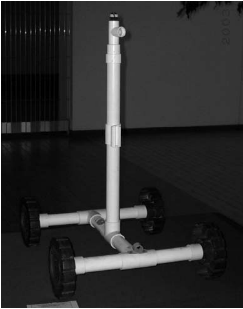
Sprinkler Stand from scrap PVC pipe
